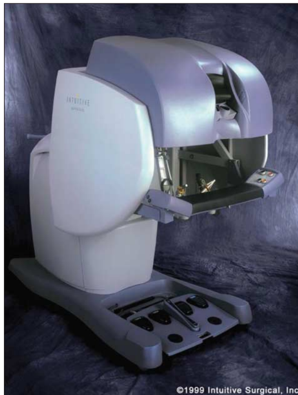
Figure 5. Surgeon's console component of the da Vinci Surgical Robot (Intuitive Surgical Inc, Sunnyvale, Calif; photograph used with permission).
